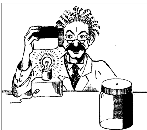
Fig. 2. Can we hear light? It is possible to hear the hum produced by an ac-powered light bulb after photoacoustic conversion. Kitchen equipment will do!
